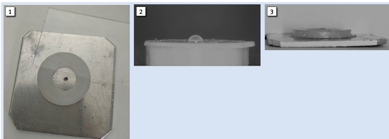
Figure 1 The Teflon mold used in this experiment is shown. It is stabilized on a metal base, and a glass slab is used to achieve flattened surface. The hole at the center denoted with an arrow was designed as an escape route for excess impression material to avoid air entrapment and subsequent bubble formation.
